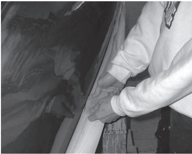
Figure 10 (bottom, right) Pushing down with the squeegee. Apply the tape a bit away from the hull.
